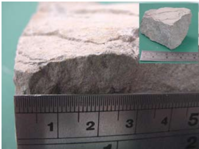
Figure 4. Typical rhyolite showing the fine-grained groundmass containing a few tiny crystals.
