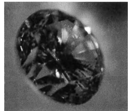
Figure 7. Photomicrograph of the .06 carat type IaAB diamond (25X magnification).
