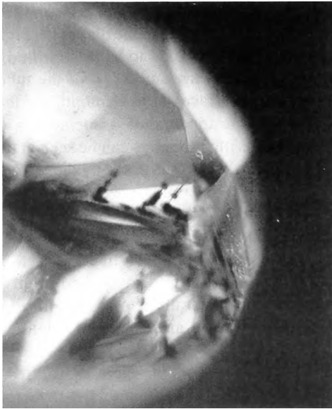
Figure 8. Photomicrograph of the radiohalos in the diamond (50X magnification).
