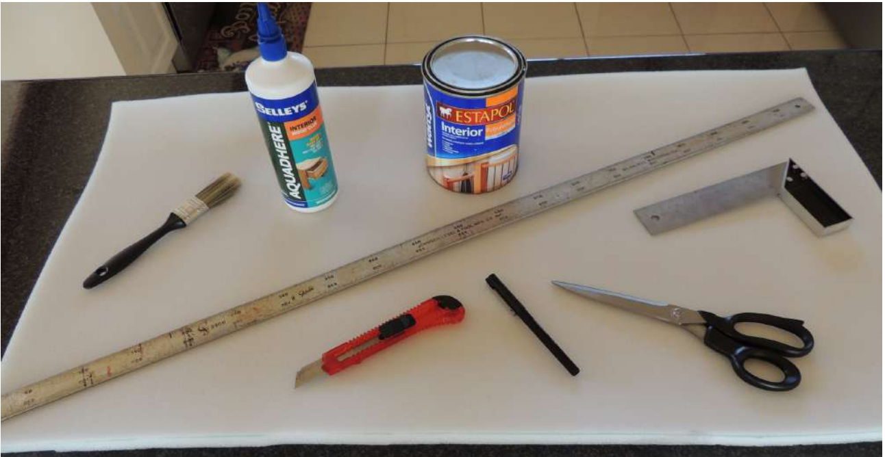
Stanley knife, scissors, long ruler, small set square, 2 litres PVA glue, 2 litres Estapol, light brown texta and small paint brush.
