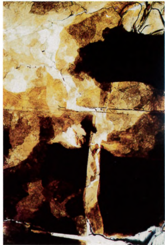
Figure 3. Photomicrograph of the same biotite in sample IM-6 after heating 250–550°C over 4 hours (63X magnification). Damage to the biotite has been considerable.
