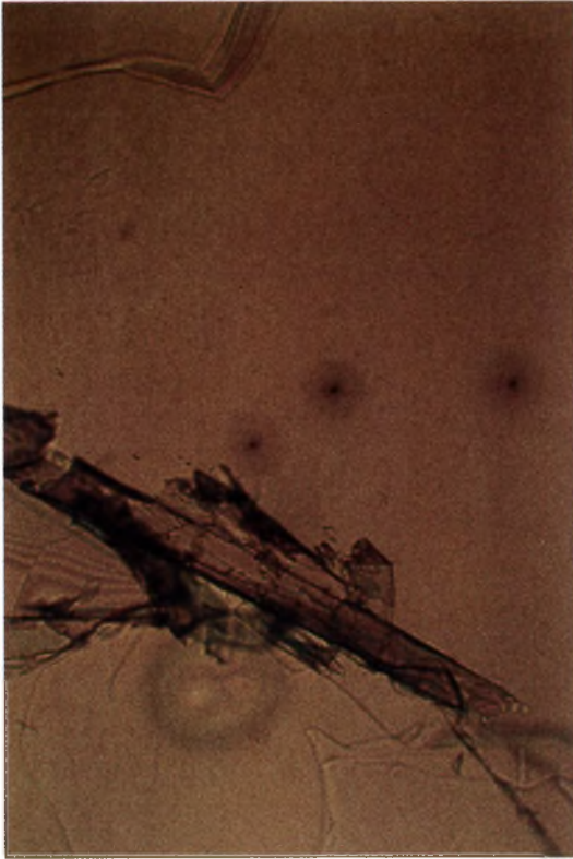
Figure 14. Photomicrograph of biotite with Po-210 radiohalos in sample BLR-1 prior to heating (125X magnification).
