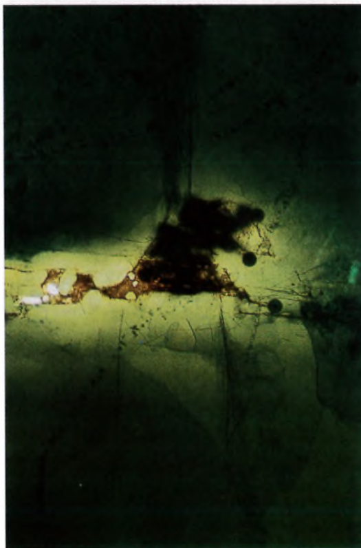
Figure 16. Photomicrograph of biotite with Po-210 radiohalos in sample IM-8 prior to heating (125X magnification).
