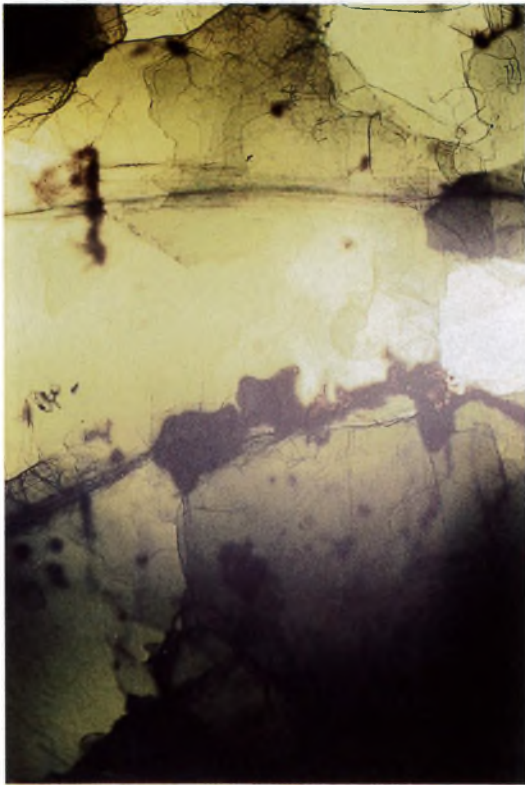
Figure 2. Photomicrograph of biotite in sample IM-6 prior to heating (63X magnification).
