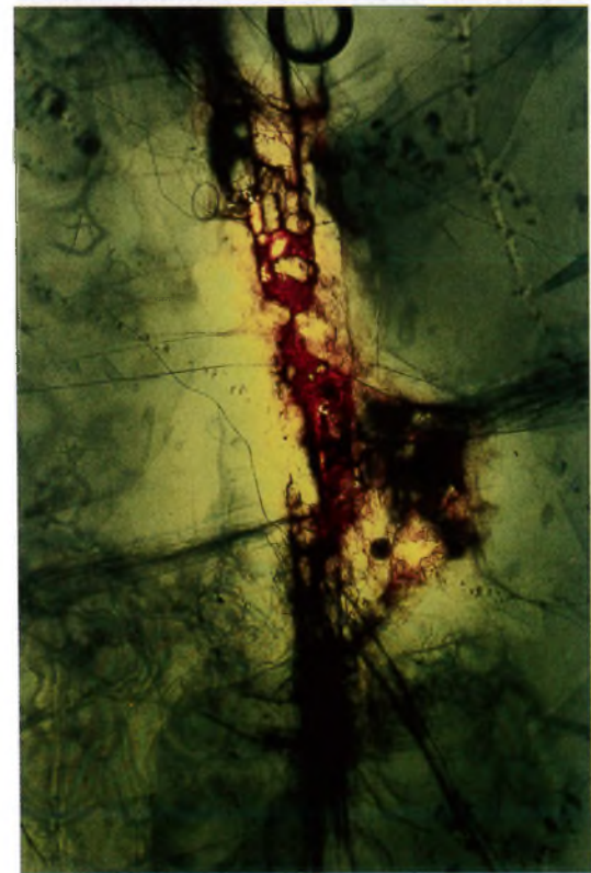
Figure 17. Photomicrograph of the same biotite in sample IM-8 after being heated at 300°C for 5 hours but the Po-210 radiohalos have been erased (125X magnification).
