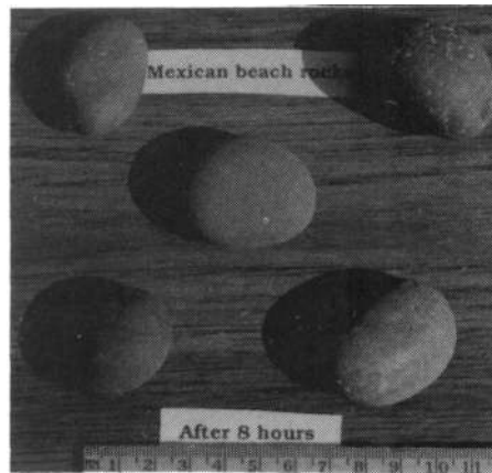
Figure 12. Metasediment (Mexican Beach Rock) samples after eight hours of erosion.
