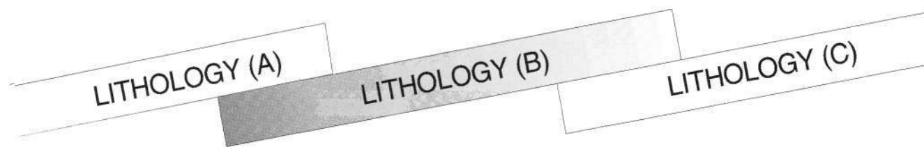
Figure 2. It has been argued that strata should be counted as stratigraphically superposed because strata can overlie each other through a series of overlaps like the tiles of a gabled roof. However, strata change in character laterally over long distances and the horizons of supposed geologic time cut across lithologies. So regional overlapping cannot be empirically counted as superposition.
