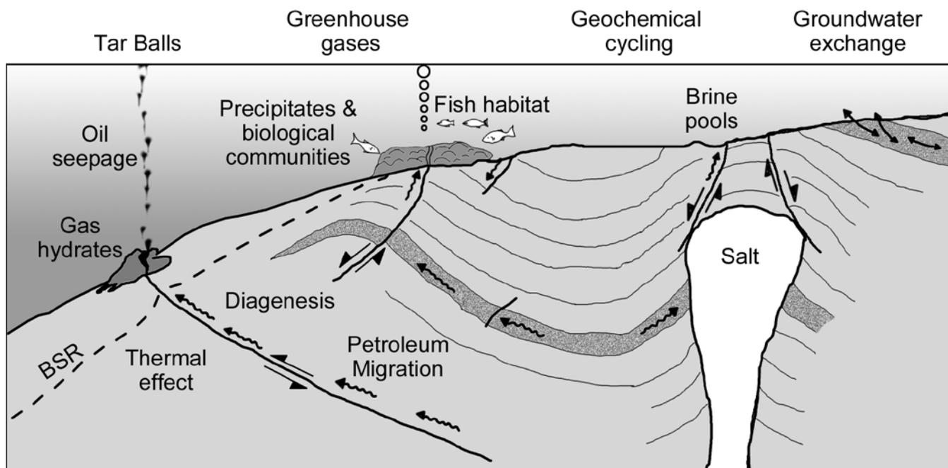
**Figure 2.** Schematic cross section of seepage system showing the role of faults, stratigraphy and salt in focusing fluid flow (BSR = boundary of saltwater regime). Seafloor manifestations of seepage include direct expulsions of oil and gas, gas hydrates, biological communities and precipitates of various types (from Moore, used with permission).<sup>3</sup>
