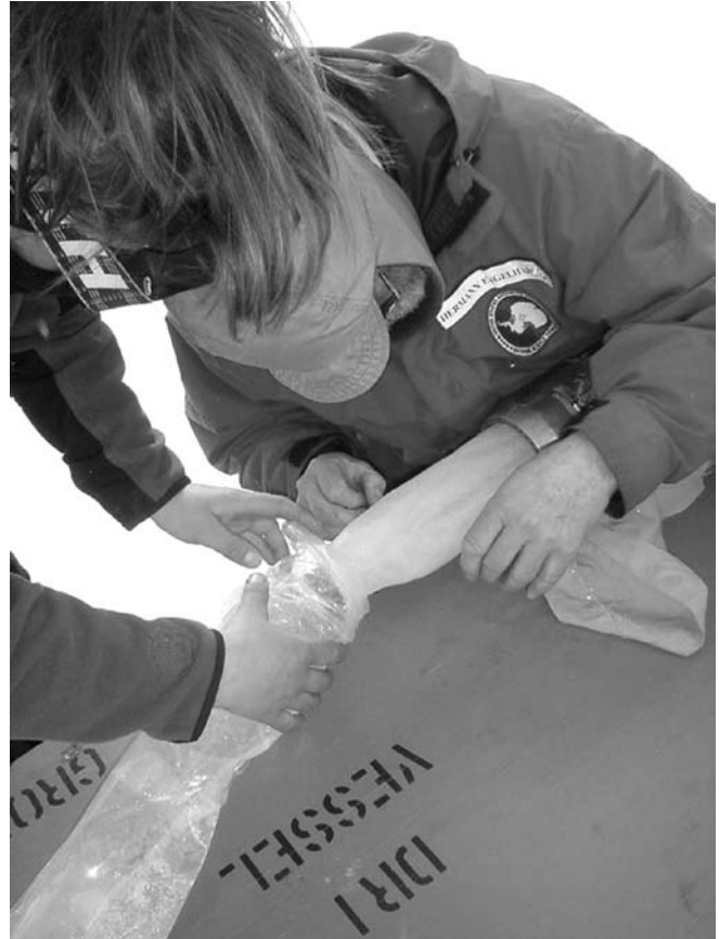
Ice cores are retrieved in short sections and transferred from the core barrel to a protective plastic sleeve.
