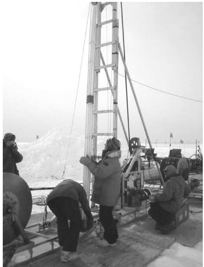
Modified drilling rigs are used to obtain ice cores.
