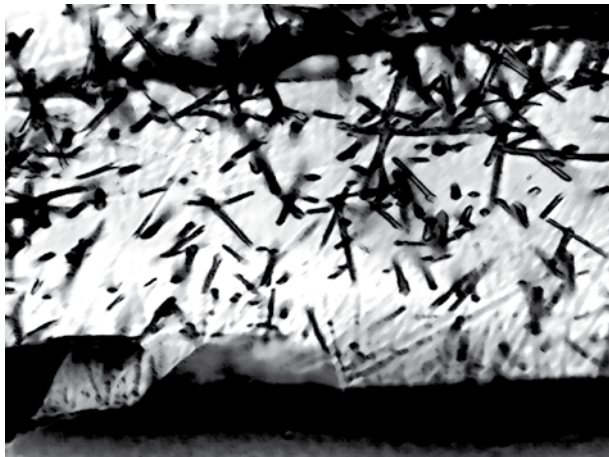
Artist's impression of fission tracks on etched and polished zircon crystal from a sample of the Peach Springs Tuff obtained from an outcrop in the Snaggletooth area of southern California close to the Arizona border.
