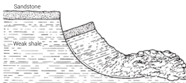
Figure 4. A rotational slump (from Foster 64 ). Notice the similarity to the ‘accretionary prism’ in figure 2.
