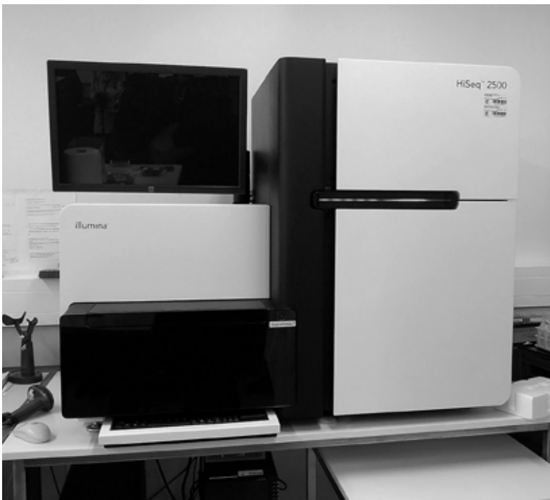
Figure 2. Illumina HiSeq 2500 DNA sequencer. This next-generation, ultra-high-throughput system can be found in major genome centres, including those that process ancient DNA. Systems like these allow researchers to move from sample preparation to whole genome sequence acquisition in just a few days.
