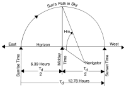
Figure 2. The relationship between the sun's maximum height angle ( H_m ), the length of day ( T_d ) and the sun's path in the sky. For September 11, 1992, H_m equals 49.3^\circ and T_d equals 12.78 hours.
